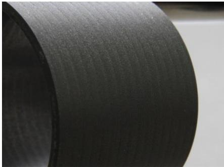
Picture 2: small, precise stack in NO20
